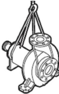
The pump-motor train must be transported as shown below:
