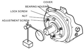
Zero the dial indicator and loosen the lock screws approximately one turn.
