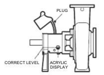
The first bearing oil change should be done after the first 200 hours of equipment operation. Afterwards, the lubricant oil changes must happen after every 2000 hours of operation or every 3 months (whichever happens first).
