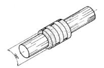
Check if the shaft can rotate after assembling each ring. Position the packing gland pressing the last ring, and manually tighten the nuts. Turn the shaft to assure that it does not touch the packing gland.
